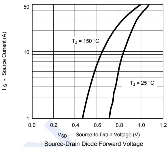
$V_{SD}$  - Source-to-Drain Voltage (V)
