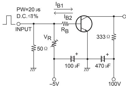
$I_C = 20I_B1 = -20I_B2 = 300\text{mA}$
